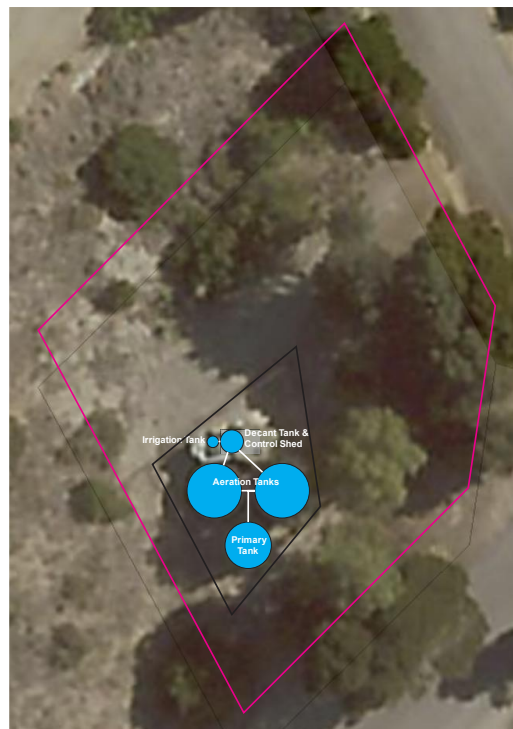
Figure 2 Treatment Plant Layout
