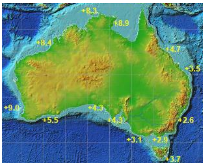
Figure 8: (Left) Australian sea level changes (mm/year) from the early 1990s when the National Tidal Centre Sea Level Rise project started to end June 2011. The measurements take into account changes due to tectonic subsidence and uplift and seasonal climatic influences (Source: National Tidal Centre 2011).
