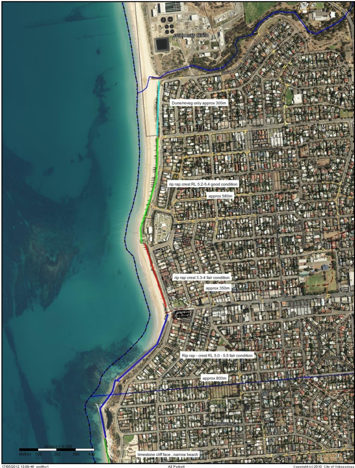
CITY OF ONKAPARINGA Christies Beach South Australia Map showing type, condition and approximate extent of coastal protection works North end This material is provided for general information only without any express or implied warranty as to its accuracy or currency. No action should be taken on the basis of this material. Appropriate independent professional advice should be obtained.
