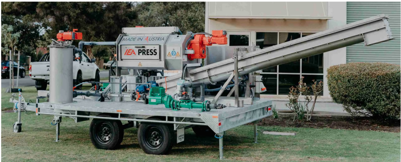
Figure 9 Mobile screw press (Source: IFS)
