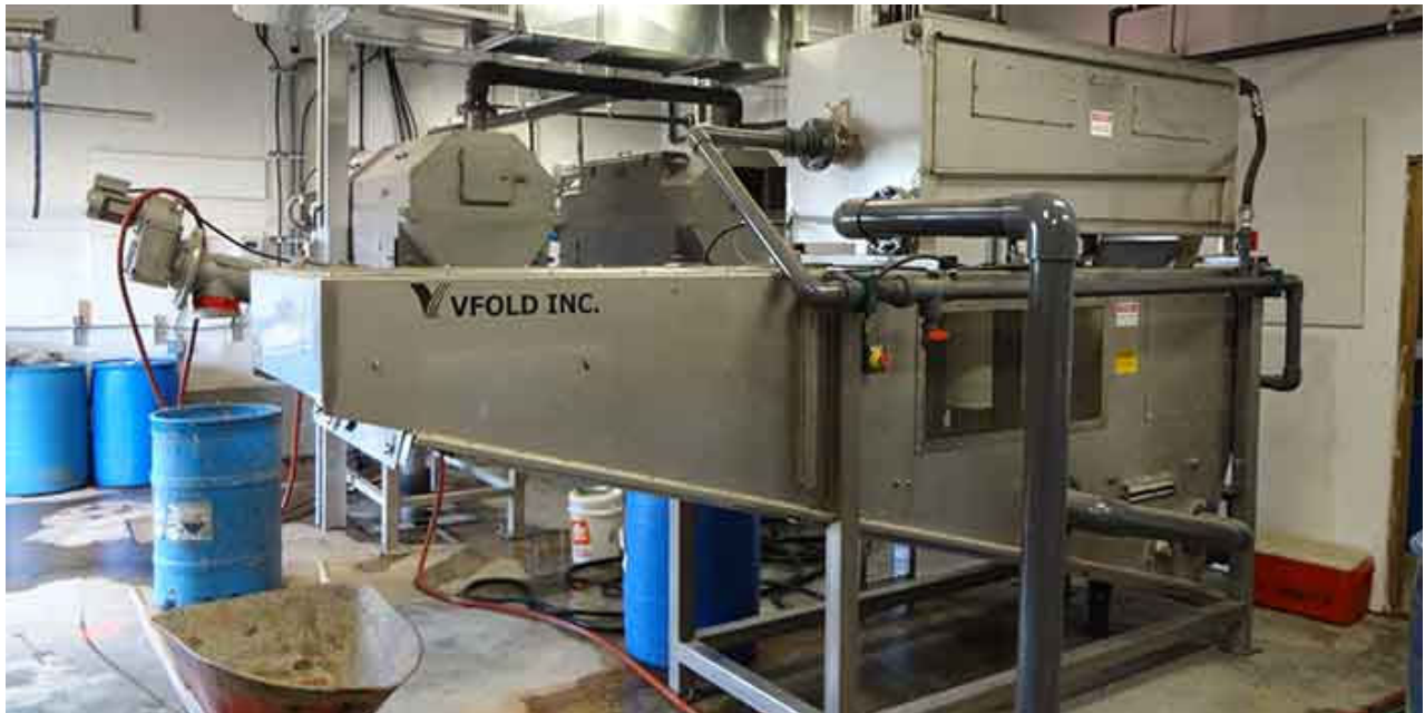
Figure 8 Typical V-Press (Credit: Vand Solutions)
